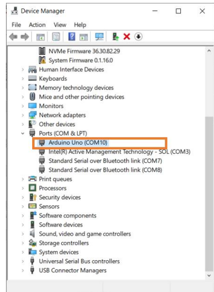
Figure 8. Device Manager window. For this example, the COM Port assigned to the Arduino UNO is the COM 10.
