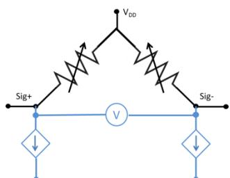
Constant Current Mode: Current level should be chosen for patient safety, signal-to-noise and lifetime requirements. (Blue portions of circuit supplied by customer.) Refer to ISO 60601 for patient risk current safety limits.
