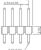
PCB thickness is 1.57mm. Straight pin, through-hole pin headers have 2.54mm pitch, 6mm mating length and 3mm termination post length.
