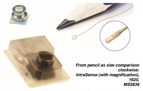
The IntraSense pressure sensor, which is only 220  $\mu$ m wide, fits into the smallest 1 French catheters. With its wide pressure range of -300..500 mmHg, it can measure blood pressure as well as intracranial or bladder pressure quickly and directly on site. For rapid initial development steps, AMSYS also offers an evaluation kit with USB connection and software for initial measurements of pressure and temperature for prototyping.
